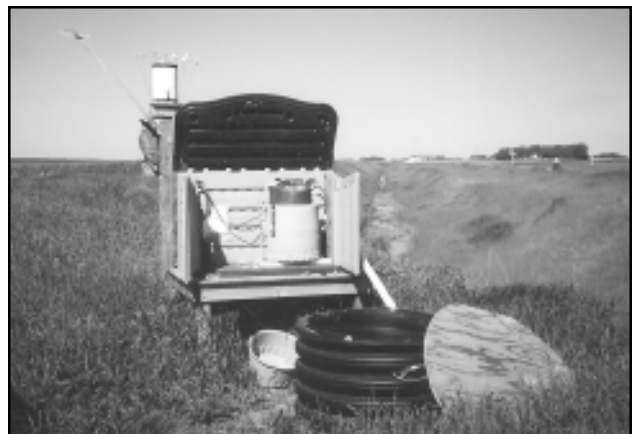
Figure 3. Automatic water monitor and sampler, ISCO 6700, with rain gauge and tile line access manhole for instrument maintenance.
